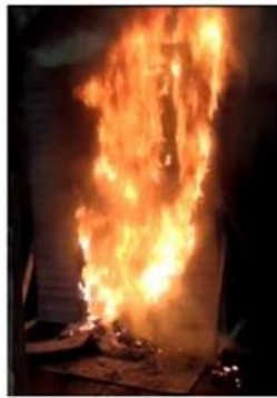
Figure 10. 6. Exp. 5 – Vinyl siding over polystyrene
