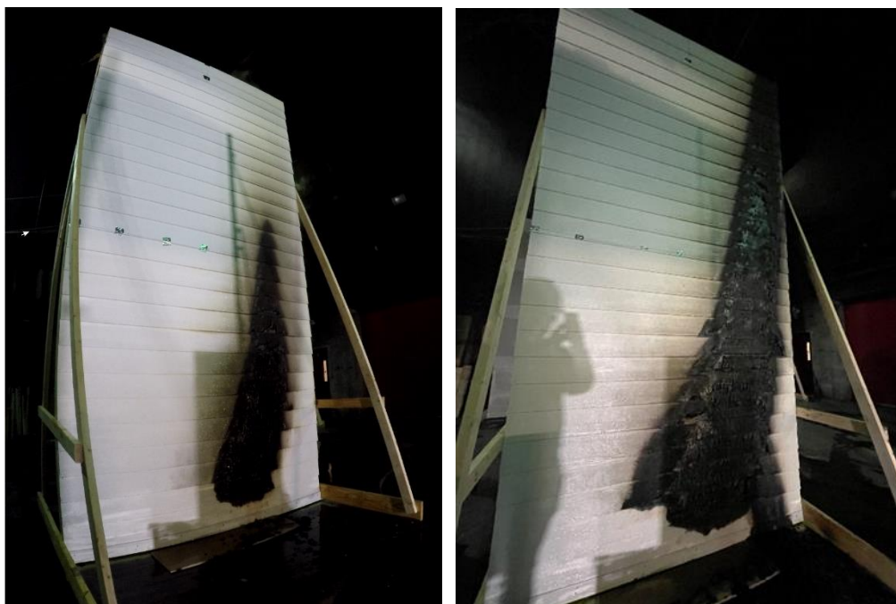
Figure 31 - 20 Minute Ignition Fire Exposure 50 kW (Left) versus 75 kW (Right)
