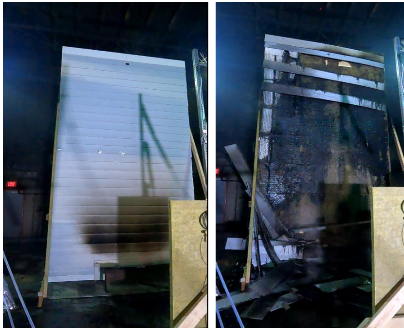
Figure 37 - Test 7 Photographs of After the First Test Exposure (Left) and After the Second Test Exposure with Fiber Cement Siding Panels Removed (Right)
