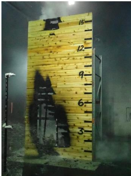
Figure 46 - Post-test Photograph of Test 7 Cedar Siding/House Wrap/Plywood Wall Assembly with 75 kW Ignition
