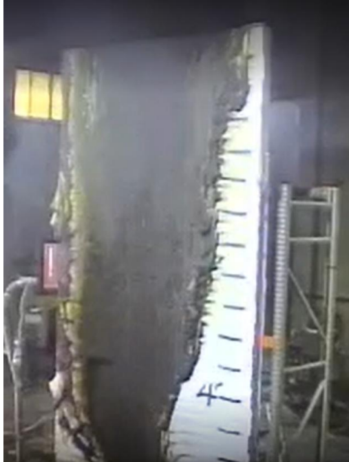
Figure 43 - Post-test Photograph of Test 4 Vinyl Siding/1 in. XPS/OSB Wall Assembly with 100 kW Ignition
