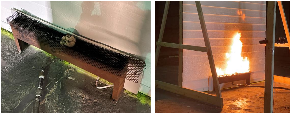
Figure 18 - Photographs of the Test Burner and 75kW Ignition Fire
