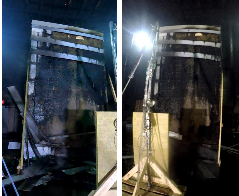
Figure 26 - Post-test Photographs of Test 7b Fiber Cement Siding/EPS/Mineral Wool Wall Assembly with 75 kW Ignition After Panel Removal
