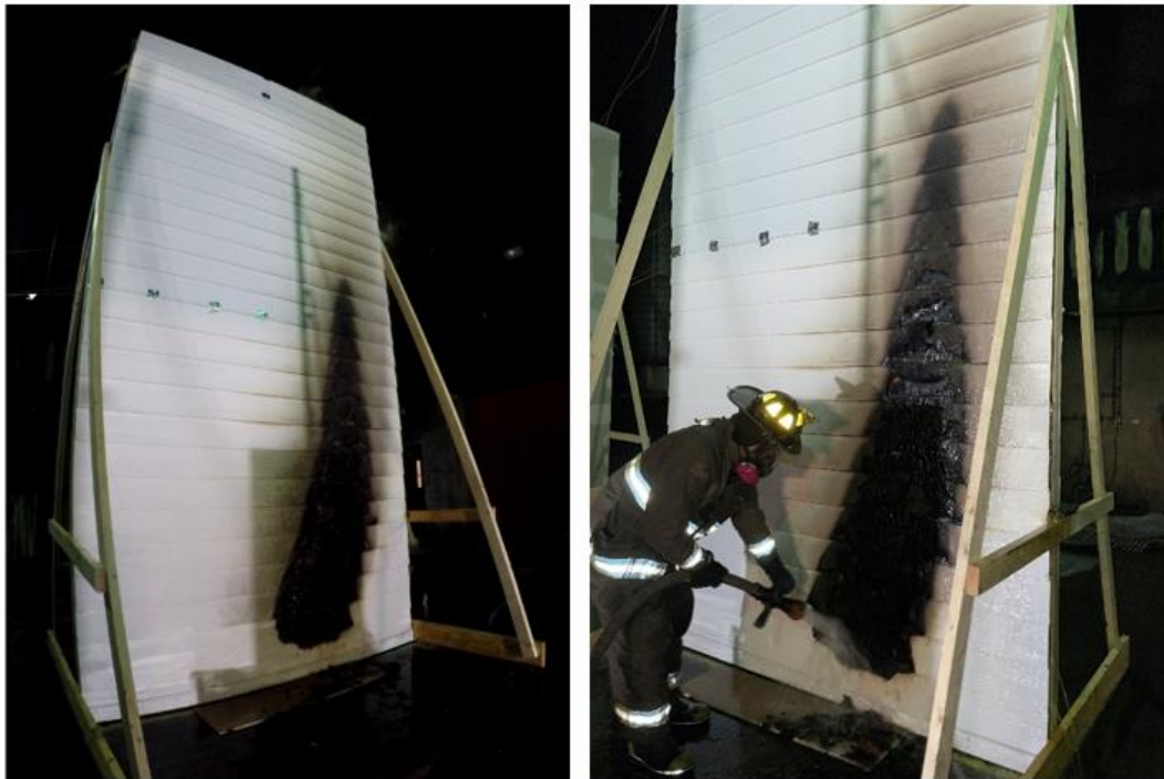
Figure 20 - Post-test Photographs of Test 2 Wood Composite Siding/Asphalt Paper Wall Assembly with 50 kW Ignition
