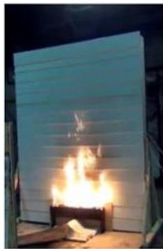
Figure 10. 8. Exp. 19 – Fiber Cement Siding
