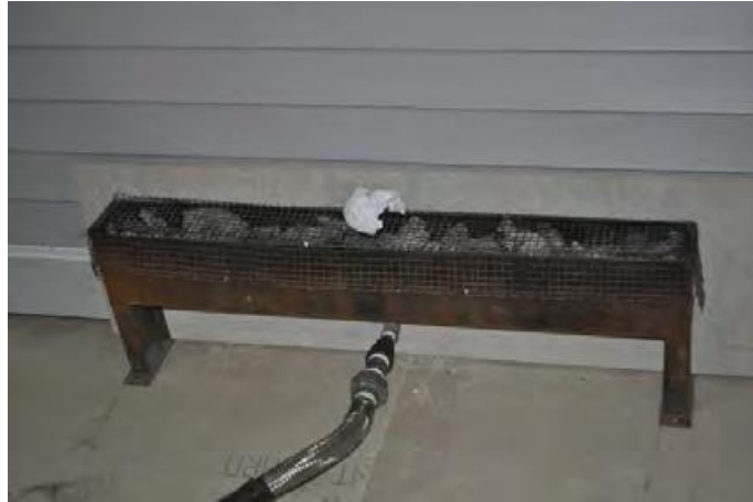
Figure 10 - Photograph of the 39 inch (1 m) Gas Line Burner [7]
