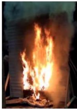
Figure 10. 5. Exp. 3 – Vinyl Siding over plywood
