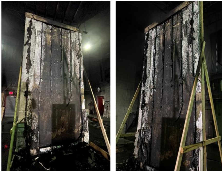
Figure 24 - Post-test Photographs of Test 6 Vinyl Siding/EPS/Mineral Wool Wall Assembly with 75 kW Ignition
