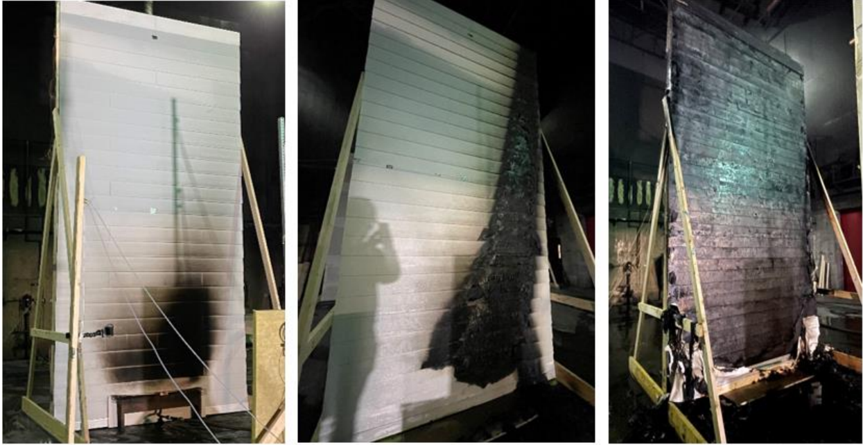
Figure 32 - Side by Side Post-test Photographs from Test 1 and Tests 3-4 of Similar Wall Assemblies with Different Siding - Fiber Cement, Wood Composite, and Vinyl (Left to Right)
