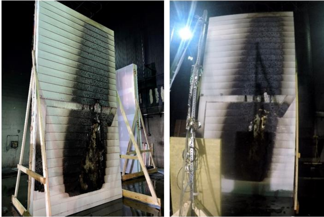
Figure 23 - Post-test Photographs of Test 5 Wood Composite Siding/EPS/Mineral Wool Wall Assembly with 75 kW Ignition
