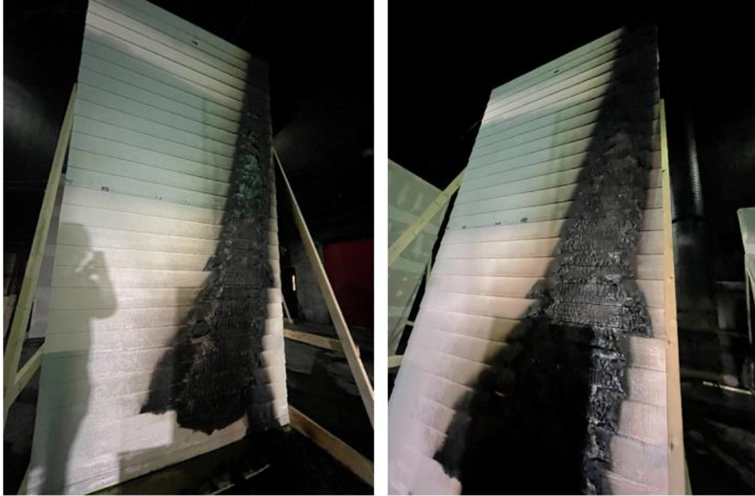
Figure 19 - Post-test Photographs of Test 1 Wood Composite Siding/Asphalt Paper Wall Assembly with 75 kW Ignition
