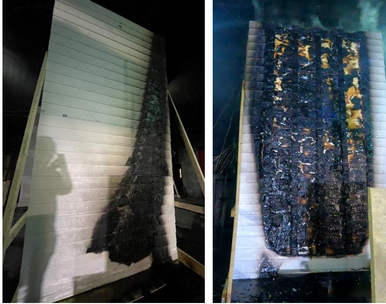
Figure 34 - Side by Side Post-test Photographs of Two Wood Composite Siding Tests (Test 1 & 10) with Differing Interior Layers
