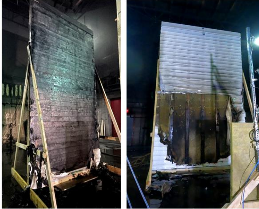
Figure 35 - Side by Side Post-test Photographs of Two Vinyl Siding Tests (Test 3 & 11) with Differing Interior Layers
