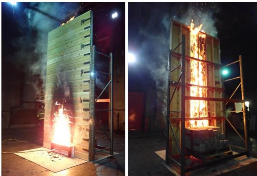
Figure 12 - Photographs of Fire Burning through Test Sample
