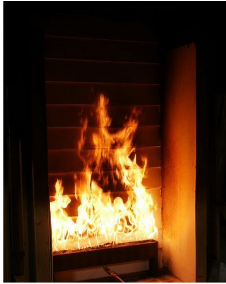
Figure 3 - Photograph of ASTM E2707 Test
