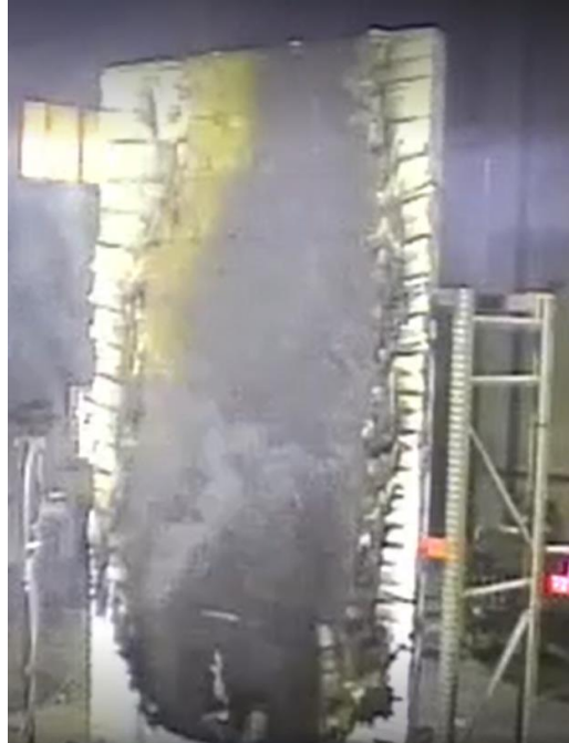
Figure 40 - Post-test Photograph of Test 1 Vinyl Siding/House Wrap/OSB Wall Assembly with 100 kW Ignition
